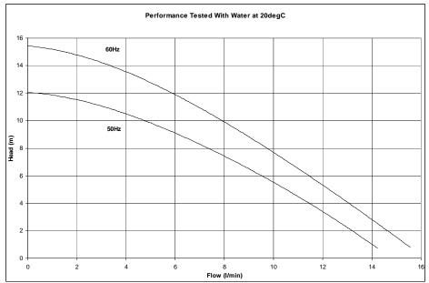
NOTE: These pumps are designed for use with clean fluids. Solids will cause jamming. Abrasives will reduce pump life & invalidate the warranty. SPC pumps are self-priming. The company reserves the right to change specifications
