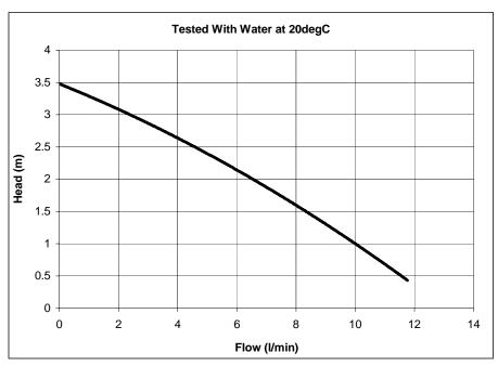
NOTE: These pumps are designed for use with clean fluids.
